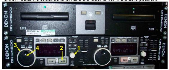
To select a track, rotate the small white knurled knob (1) until the correct track number shows.
